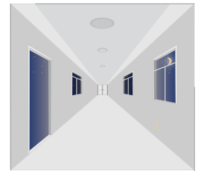
The sensor turns OFF light automatically after the standby period when there' s no motion detected.
